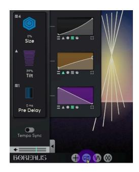
By clicking the expand icon (four corners), you can enlarge the tables for fine-tuning or to access the preset table shapes, including a randomizer. This feature allows for more precise control and customization of the parameters, ensuring that you can achieve the exact response you desire.
