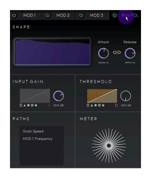
Additionally, you can adjust the envelope follower input gain and open the envelope follower page using the designated slider and icon on the front page for easy access.
