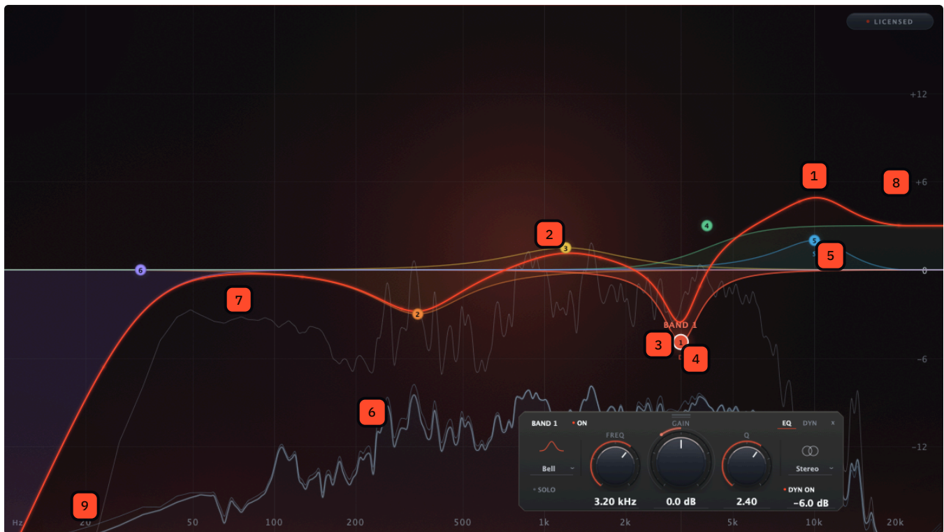
FIG. 2 The EQ display: the summed curve in ember, each band in its own color, and the analyzer underneath.
