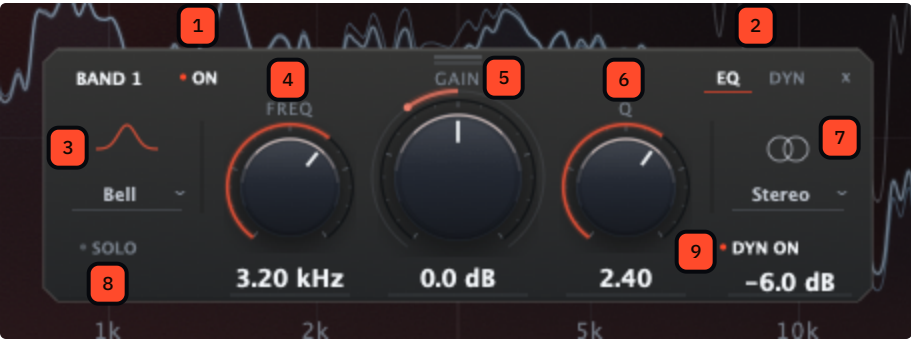
FIG. 4 The EQ page for band 1, a dynamic bell at 3.2 kHz.
