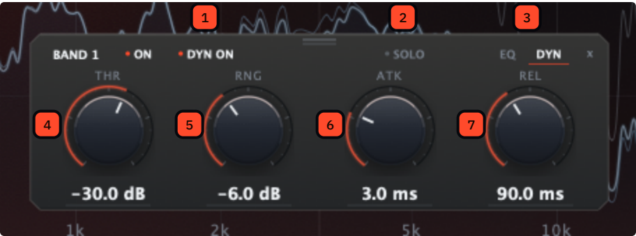
FIG. 6 The DYN page for the same band: threshold, range, attack and release.
