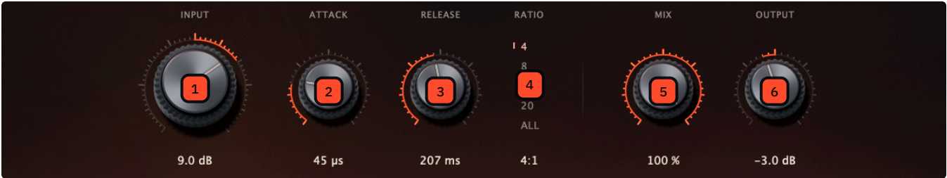
FIG. 4 FET mode: input, attack, release, the ratio values, mix and output.
