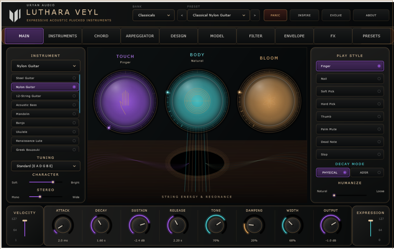
The Main page with the persistent header, page navigation, performance panel, three macro orbs, and bottom control strip.
