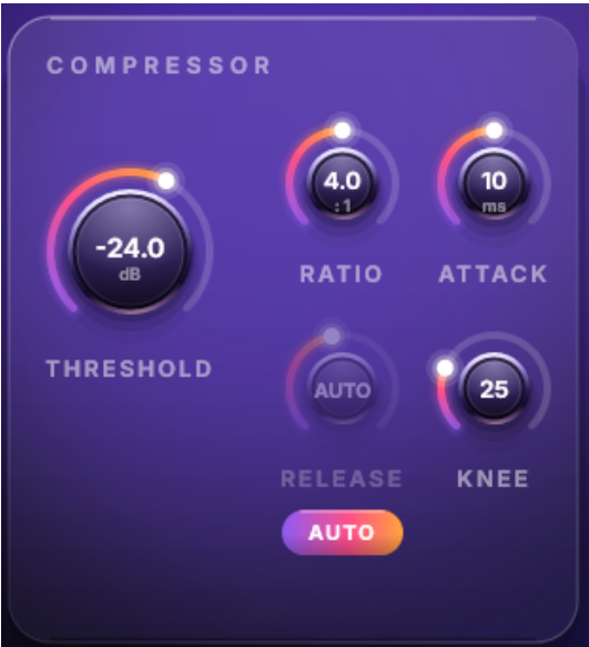
AUTO REL on. The RELEASE knob is disabled.
